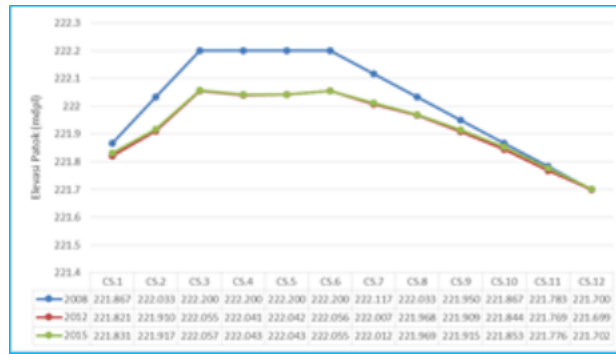
Figure 11. Settlement at the top of the dam during the Big check
